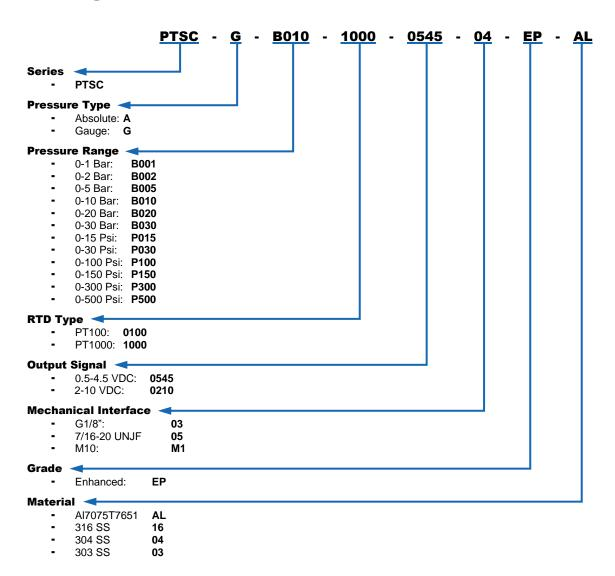
Typical ordering example: Gauge, 10 bar pressure, PT1000 RTD, 0.5-4.5 output signal, M10 mechanical interface, Enhanced grade, Al7075T7651 material: PTSC-G-B010-1000-0545-M1-EP-AL
