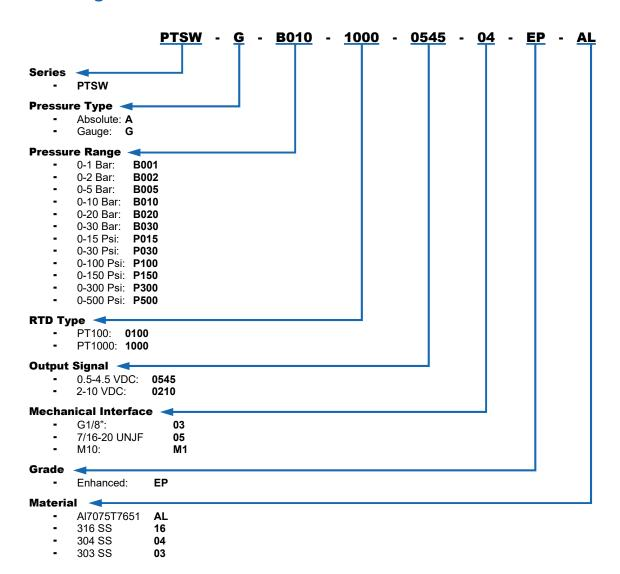
Typical ordering example: Gauge, 10 bar pressure, PT1000 RTD, 0.5-4.5 output signal, M10 mechanical interface, Enhanced grade, Al7075T7651 material: **PTSW-G-B010-1000-0545-M1-EP-AL**
