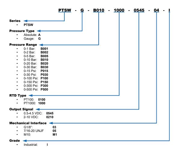
Typical ordering example: Gauge, 10 bar pressure, PT1000 RTD, 0.5-4.5 output signal, M10 mechanical interface, Industrial grade: PTSW-G-B010-1000-0545-M1-I
