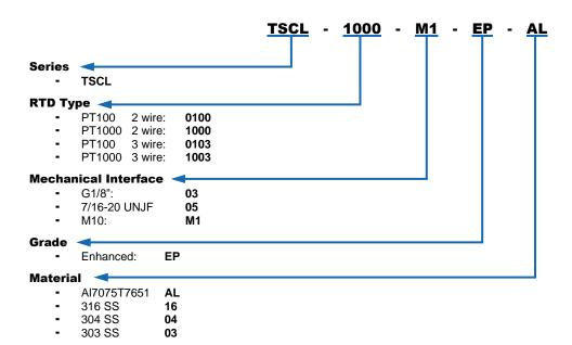
Typical ordering example: PT1000 RTD, M10 mechanical interface, Enhanced grade, Al7075T7651 material: **TSCL-1000-M1-EP-AL**
