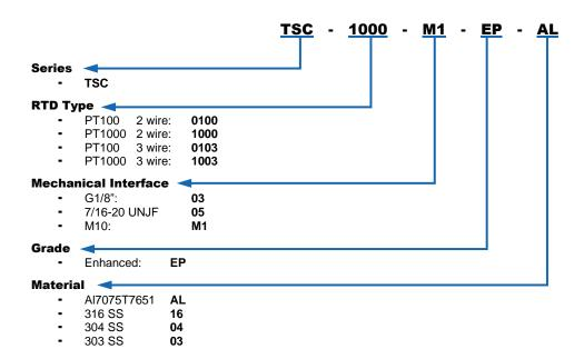
Typical ordering example: PT1000 RTD, M10 mechanical interface, Enhanced grade, Al7075T7651 material: **TSC-1000-M1-EP-AL**
