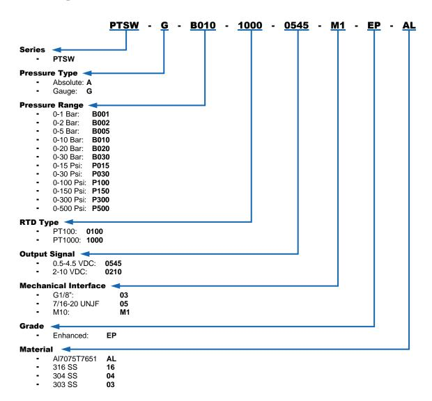
Typical ordering example: Gauge, 10 bar pressure, PT1000 RTD, 0.5-4.5 output signal, M10 mechanical interface, Enhanced grade, Al7075T7651 material: **PTSW-G-B010-1000-0545-M1-EP-AL**
