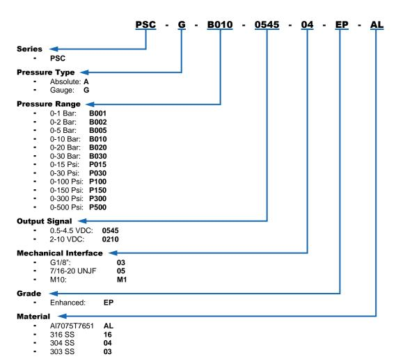
Typical ordering example: Gauge, 10 bar pressure, 0.5-4.5 output signal, M10 mechanical interface, Enhanced grade, Al7075T7651 material: **PSC-G-B010-0545-M1-EP-AL**
