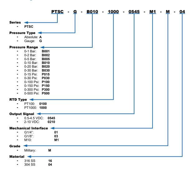
Typical ordering example: Gauge, 10 bar pressure, PT1000 RTD, 0.5-4.5 output signal, M10 mechanical interface, Military grade, SS 304 material: **PTSC-G-B010-1000-0545-M1-M-04**
