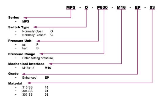
Typical ordering example: Normally open, 600 PSI pressure, M16x1.5 mechanical interface, Enhanced Grade, 303 SS material, 10cm lead wire as standard: MPS-O-P600-M16-EP-03
