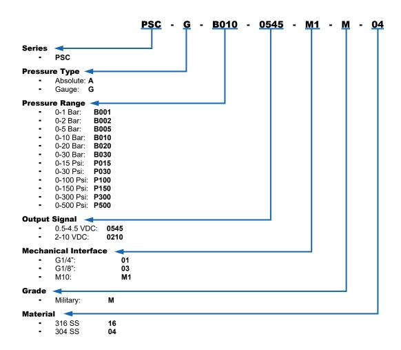
Typical ordering example: Gauge, 10 bar pressure, 0.5-4.5 output signal, M10 mechanical interface, Military grade, SS 304 material: **PSC-G-B010-0545-M1-M-04**
