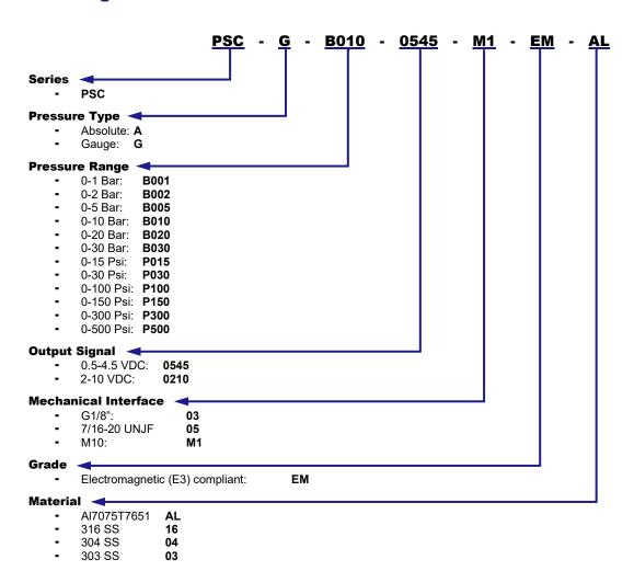
Typical ordering example: Gauge, 10 bar pressure, 0.5-4.5 output signal, M10 mechanical interface, Electromagnetic (E3) compliant grade, Al7075T7651 material: **PSC-G-B010-0545-M1-EM-AL**
